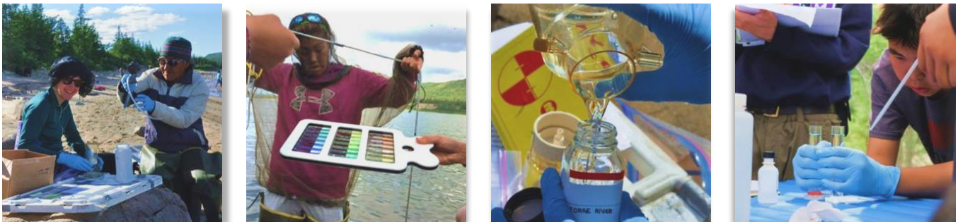
Figure 6. From left to right: water sample collection with Justine and Joshua; water color determination with Lise; water sampling for laboratory analyses; and manual measurements of turbidity with Morgan.
